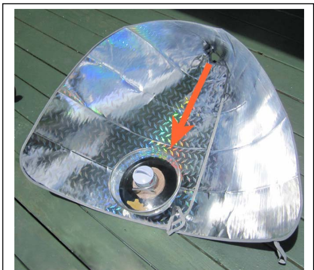
Figure 10, car shade cooker with cooking pot moved forward to track focal point.
