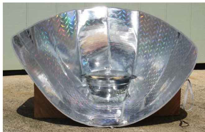
Figure 7, a cooker made from a high quality sunshade. Photo by Erik Burton
