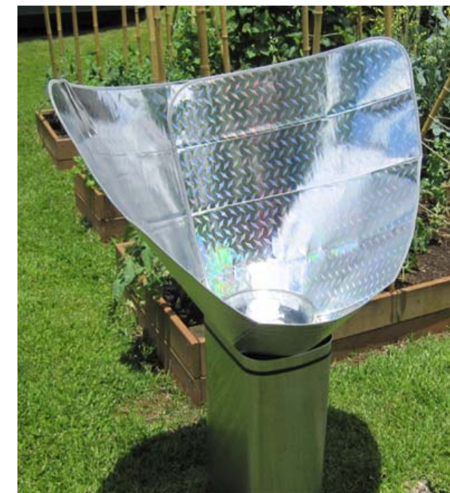
Figure 8, a cooker made from a high quality sunshade. Photo by Erik Burton
