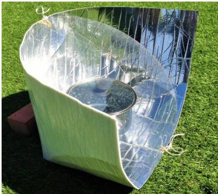
3. When the sun is low, move the cooking pot forward a few inches to tilt the cooker downward so that the front is on the ground, and the back is raised. A brick under the back will insure that the back tilts forward. This will focus more low sunlight on the cooking pot.
